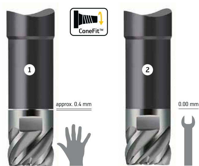
Cutter head fitting torques
