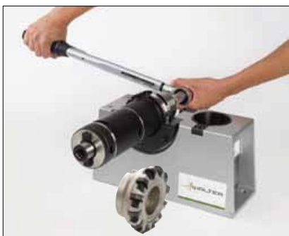
10. Tighten with a torque wrench.
