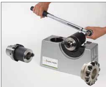
7. Tighten with a torque wrench.
