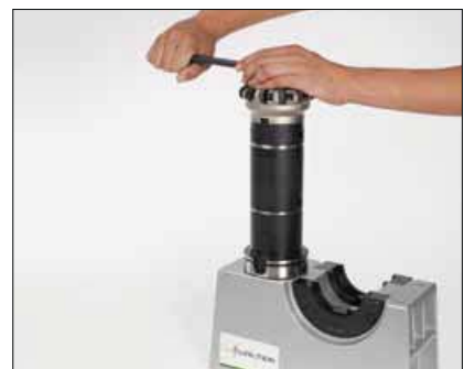
12. Install and tighten the cutting tool.
