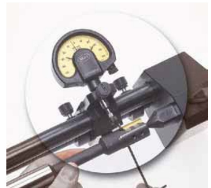
8. Measuring point B: set gauge on guide rail to 0 (similar to point 6). Then set the insert to a diameter where a taper of 1 \mu\text{m} per mm of cutting length is achieved.
