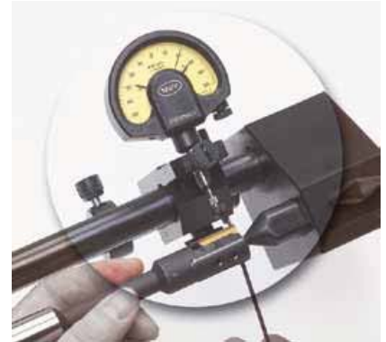
7. Measuring point A: Set the insert using adjusting ① screw so that the cutting edge is 0.02/0.015 mm above the guide pad (see picture below). This setting corresponds with the diameter marked "SD" on the tool body.
