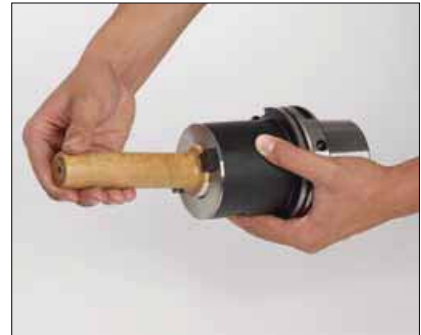
3. Clean the inside taper and the support face.
